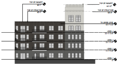
6 ELEVATION - EXTERIOR - SOUTHWEST SHORT (A3.02) 1/16" = 1'-0"
